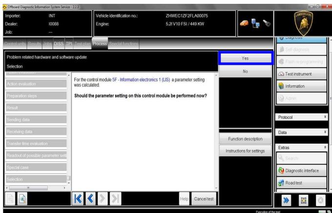
26. Wait the completion of the parameterization: at the end you'll note a reset of the MMI lasting about 1 minute.
