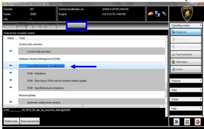
35. Execute the program “Erase fault memory – overall system” clicking on “Perform test...”
